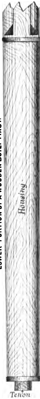
LOWER-PORCION OF A WOODEN BUILT MAST.
